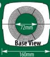
DOWNLIGHT GUARD MODEL No. I 721 72mm Cut-out Trim up to 114mm (2 piece assembly)
