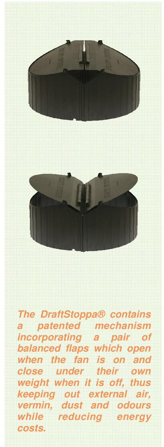
**The DraftStoppa® contains a patented mechanism incorporating a pair of balanced flaps which open when the fan is on and close under their own weight when it is off, thus keeping out external air, vermin, dust and odours while reducing energy costs.**
